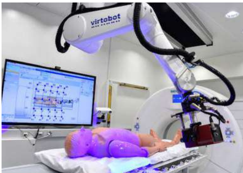
Fig. 4 A representative image of the VIRTROBOT system. Courtesy: Louise Murray, Biomedical Picture of the Day (BPoD). Managed by the MRC London Institute of Medical Sciences
