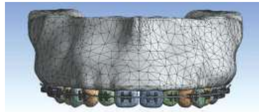
Fig 1. FEM Model of Maxilla with brackets and archwire
