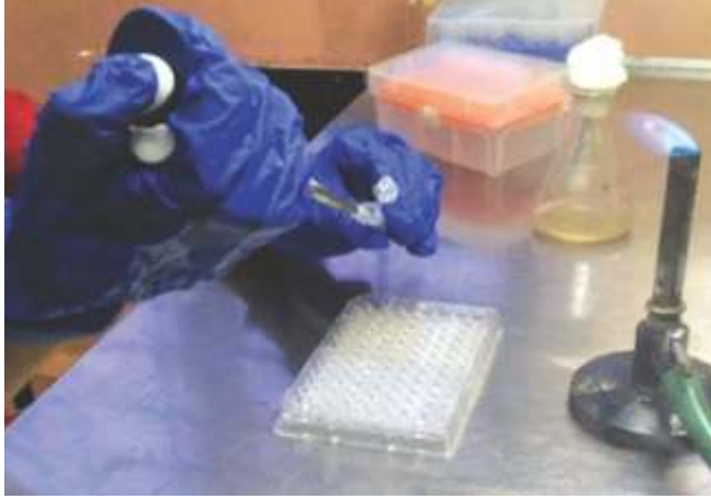
Figure 1: Pipetting the test materials into the wells
